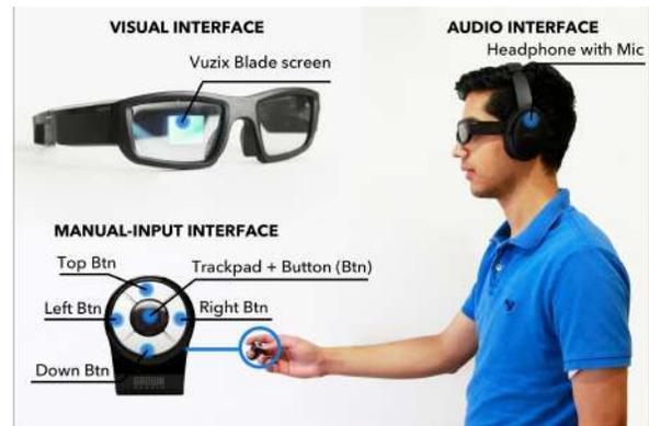
Figure 2: Apparatus showing all three interfaces.
