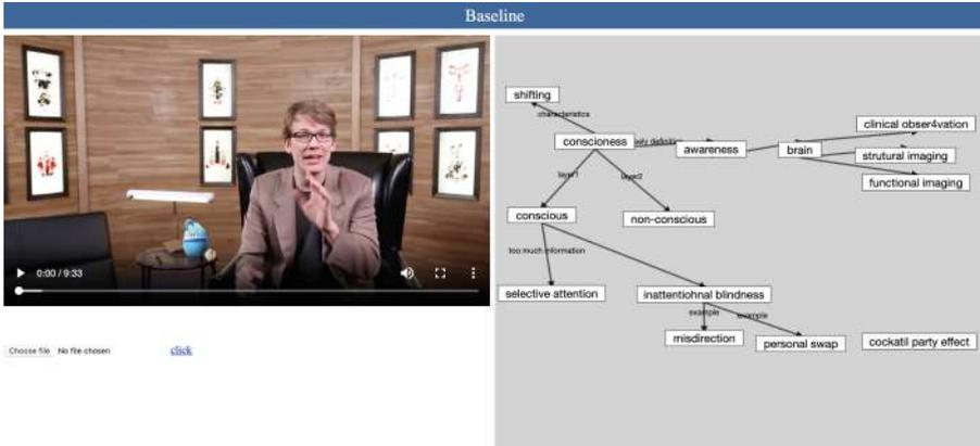
**Fig. 1.** An example concept map created by P5. The rectangle nodes represent concepts and the directed edges represent the relations. The baseline system interface consisting of a video player and a canvas. Users can create concepts, links and link labels on the canvas.
