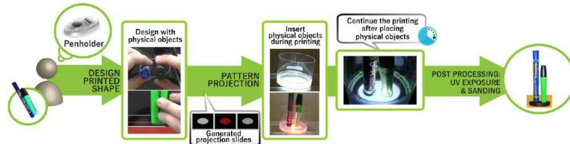
Figure 1: FusePrint fabrication process. User wants to create a penholder; its shape is designed with the reference of physical objects, and projected through the bottom of the container holding the resin and physical objects (pens). The projected shape solidifies, resulting in being perfectly matched to the objects.
