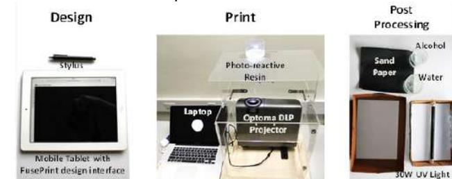
Figure 2: FusePrint Setup
