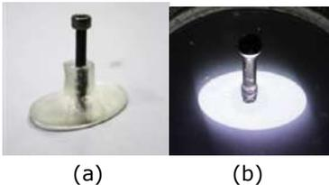
Figure 4: Print a screw thread (a) a physical screw is placed in the resin to create the internal structure for a thread (b) the screw can tightly fit into the thread
