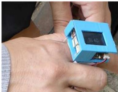
Figure 4. Ring displaying the time in standalone mode.
