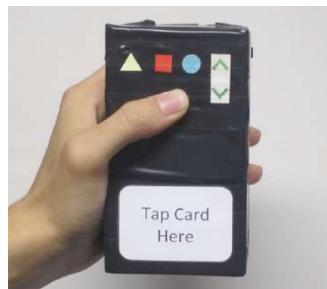
Figure 1. Elders' trigger interface in our CoFaçade prototype, with five programmable button triggers on top and a reader for RFID card triggers on the bottom. Implemented with Arduino for less than US$ 50.
