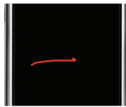
Figure 2b. ‘Tail’ generated by lifting up the right thumb after performing a left-to-right swipe motion.
