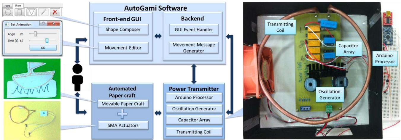
Figure 5: Overview of AutoGami's hardware and software
