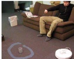
Fig. 8. Visual Feedback on Laser Trajectory
